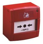
The XP95® Manual Call Point has been designed to operate on a loop of intelligent fire detection devices and when activated interrupts the polling cycle for a very fast response. The XP95 Manual Call Point is intended for indoor applications and is available in two versions, with and without isolator.
